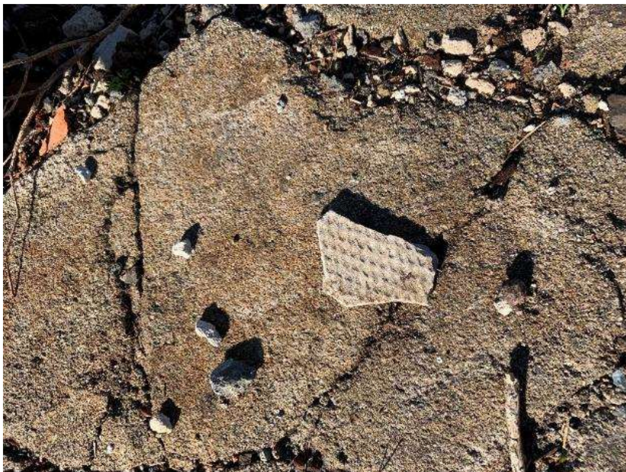
Image 6.10.1 View of fibrous cement fragment observed within building waste (brick/concrete) stockpile 5
